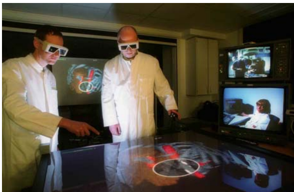
Fig. 2: Surgical Table: a special Cooperative Medical Workbench (CMW) for surgical training. Here: BERTA software module (3-D reconstructions of real radiological patient data), combined with live video conferencing for teleradiological consultation
