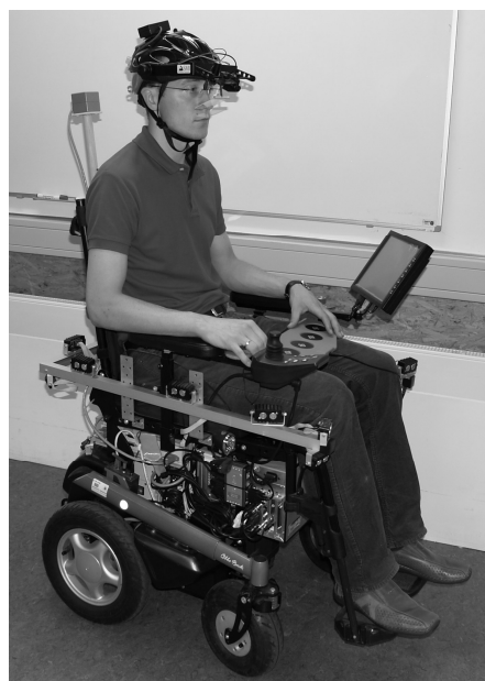
Fig. 1: Wheelchair prototype with head-mounted eye tracking device and collision avoidance sensors
