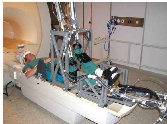
Fig. 1: The fMRI compatible robotic stepping actuator MARCOS in the 1.5T MR scanner.
