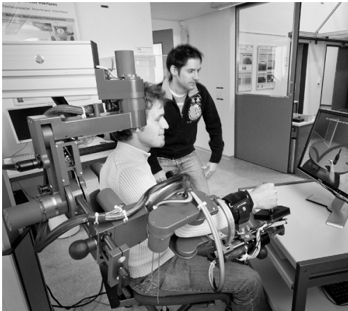
Figure 1: ARMin IV - Arm rehabilitation robot optimized for the use with SCI patients
